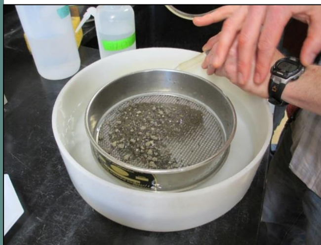
Separation of soil into water-stable aggregates using wet-sieving method
